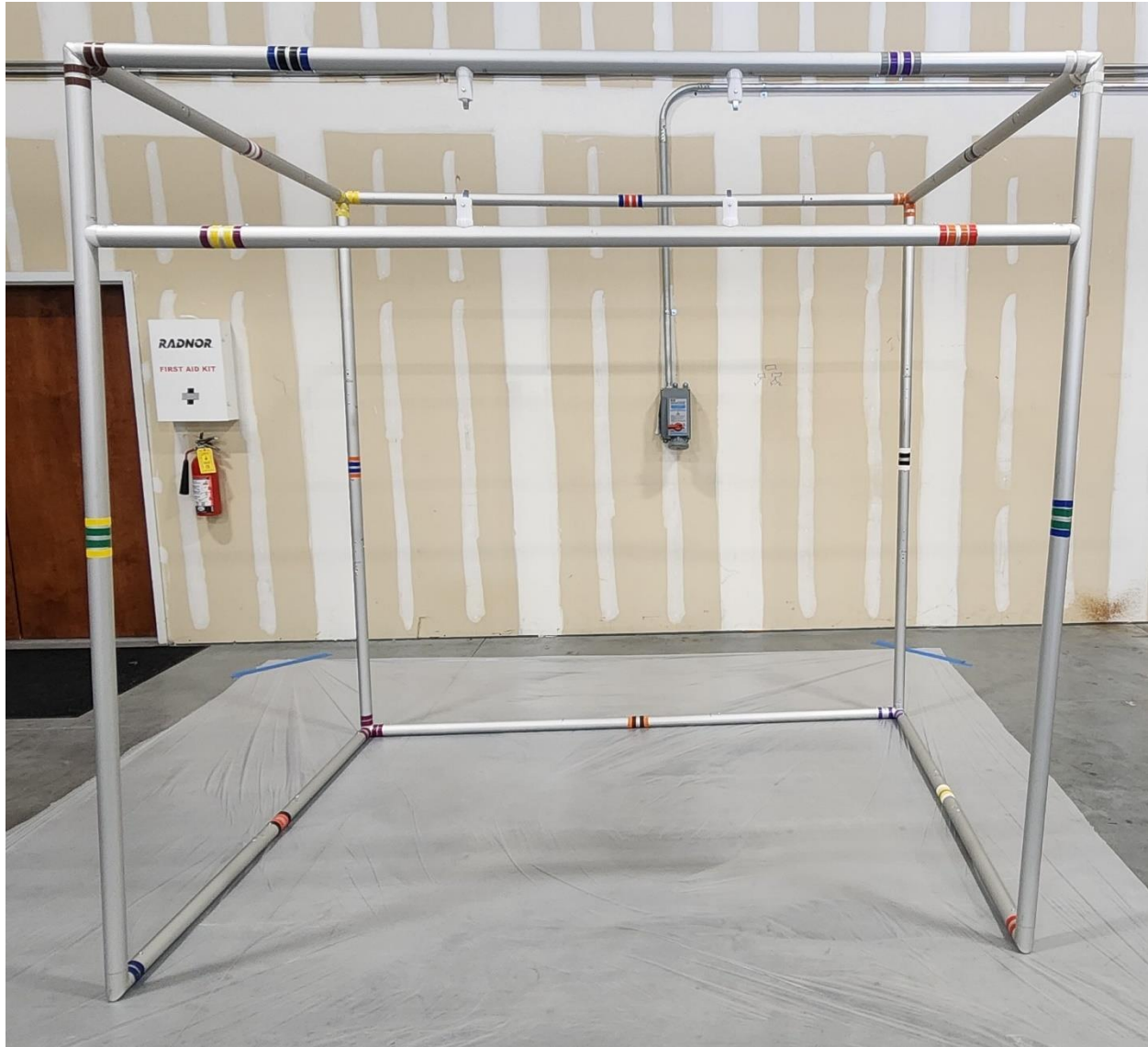
Top and Bottom Corners- Single Tape Color (single refers to 1 stripe on each part)
